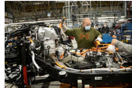
Wiring Harness Installation
